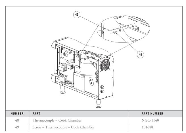
FIGURE 47: Removing the Cook Chamber (CC) Thermocouple
